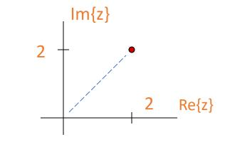
**Solution**: The path of integration is a line z = x + jy where x = y = t = [0, 2].
