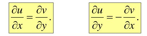
are called the *Cauchy-Riemann* equations. These equations are the criteria for a complex function to be differentiable (with respect to z = x + jy).
